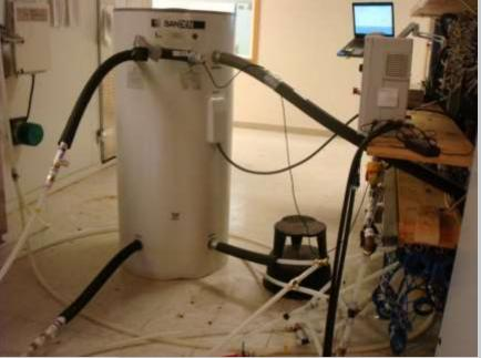
Outdoor unit in the controlled test chamber. The fluid lines connecting this to the tank are filled with potable water. Indoor tank instrumented in laboratory
